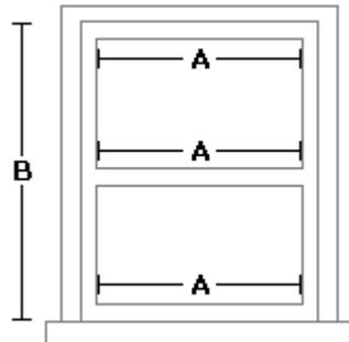
Measure inside surfaces of frame - top, middle and bottom, and use the narrowest width. Same with height - left, middle, right.
